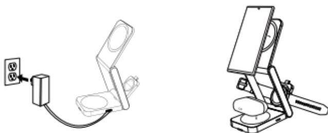
1. Connect the wireless charging station to a power source using the adapter.
